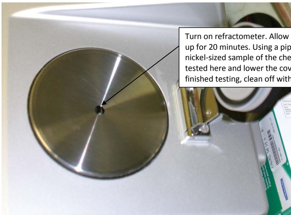
Turn on refractometer. Allow it to warm up for 20 minutes. Using a pipette, place a nickel-sized sample of the chemical to be tested here and lower the cover. When finished testing, clean off with a Kim wipe.
