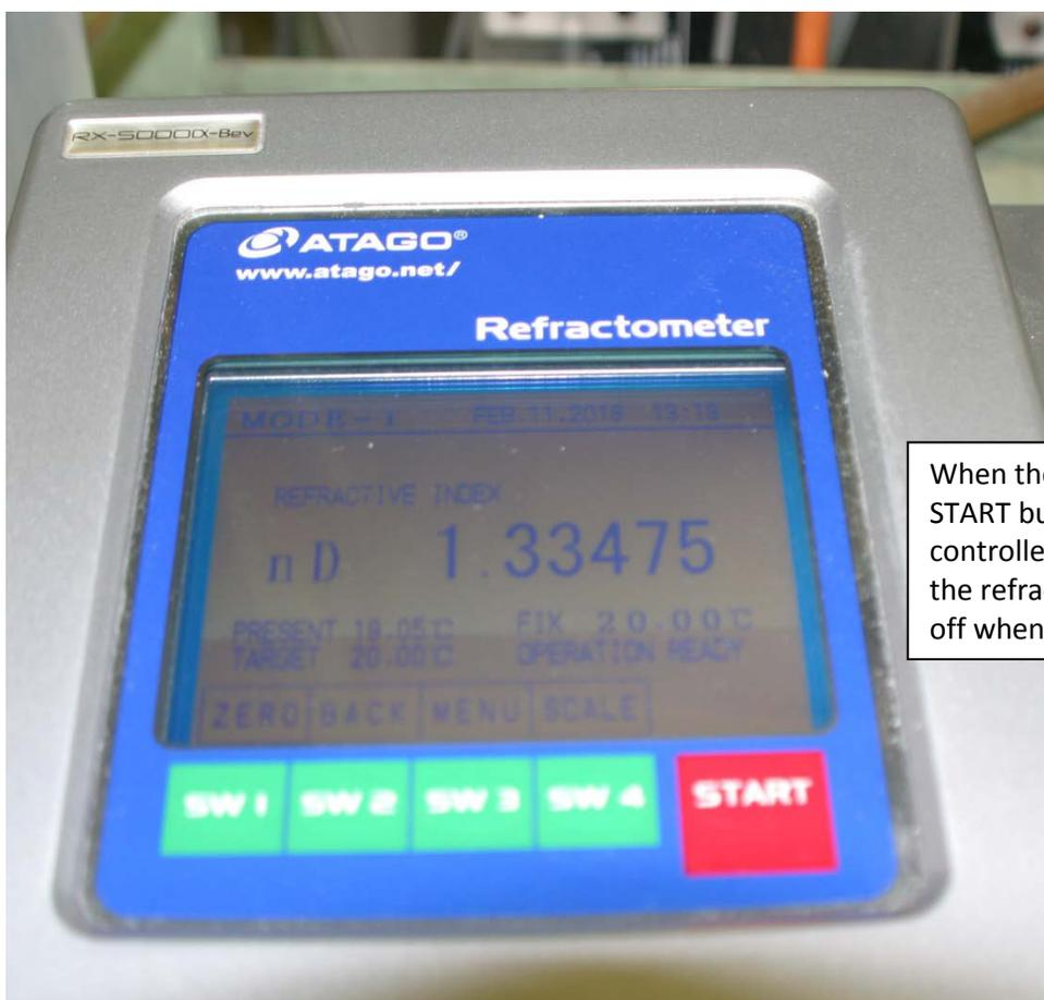
When the sample is placed, press the red START button. The temperature will be controlled. The number listed after nD is the refractive index for the sample. Turn off when done using for the day.
