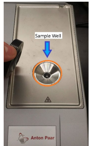
Figure 3 Sample well on the refractometer.
