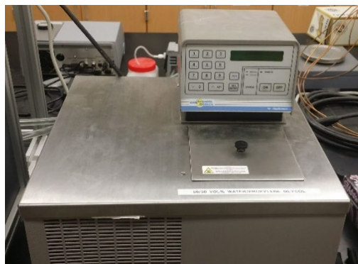
Figure 5 Refrigeration unit for chilled condenser fluid
