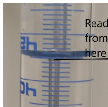
Figure 3 Meniscus of a transparent burette and where to read the fluid level.
