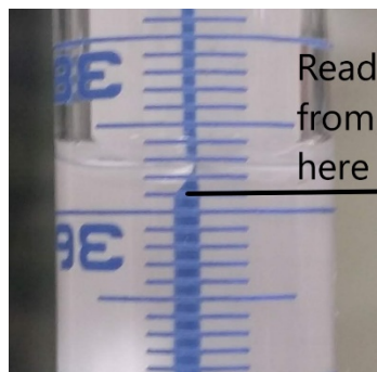
Figure 4 Meniscus of a burette with a white background and where to read the fluid level.
