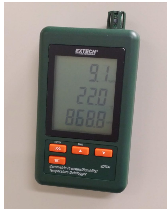
Figure 5 Ambient conditions meter located on the south fume hood.
