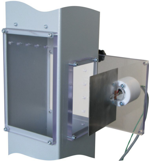
Fig. 5.7 Positioning of the plate for free convection
