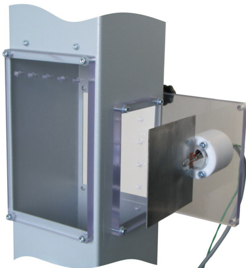
Fig. 5.2 Positioning of the plate for free convection
