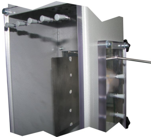
Fig. 5.16 Measuring across the flow. White blobs of thermal paste can be seen on the plate
