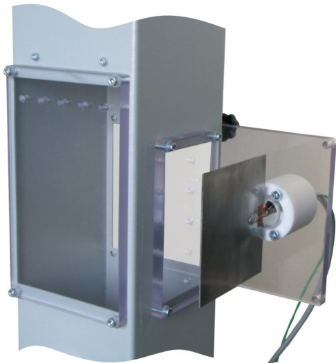
Fig. 4.6 Positioning of the heater for free convection, see Chapter 3.7.2, Page 25
