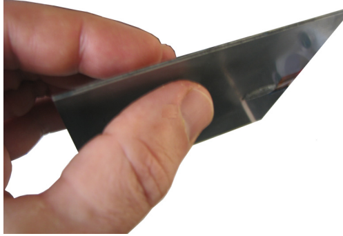
Fig. 5.3 Feeling the heat at the surface of the plate - without touching
