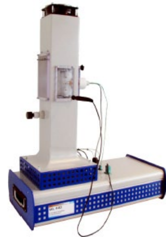
Figure 2 WL 440 Apparatus setup for forced convection
