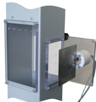
Figure 1 Apparatus setup for free convection
