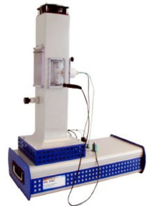
Figure 1 Experimental apparatus for measuring convective heat transfer coefficients.
