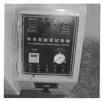
8. Turn on the SPRAY switch. Adjust the PRESSURE VALVE to 1kg/cms
