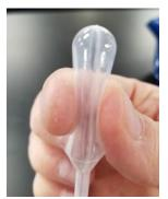
c. Remove the pipette from the beaker, while holding the tip downward and suspended above the beaker to catch any liquid. Make
